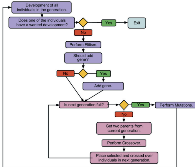
Figure 4: flow chart of the proposed framework for incremental evolution of genome representations.
