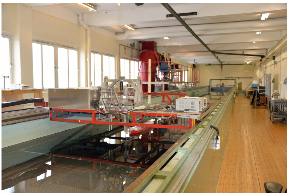
Figure C.3: The small towing tank
