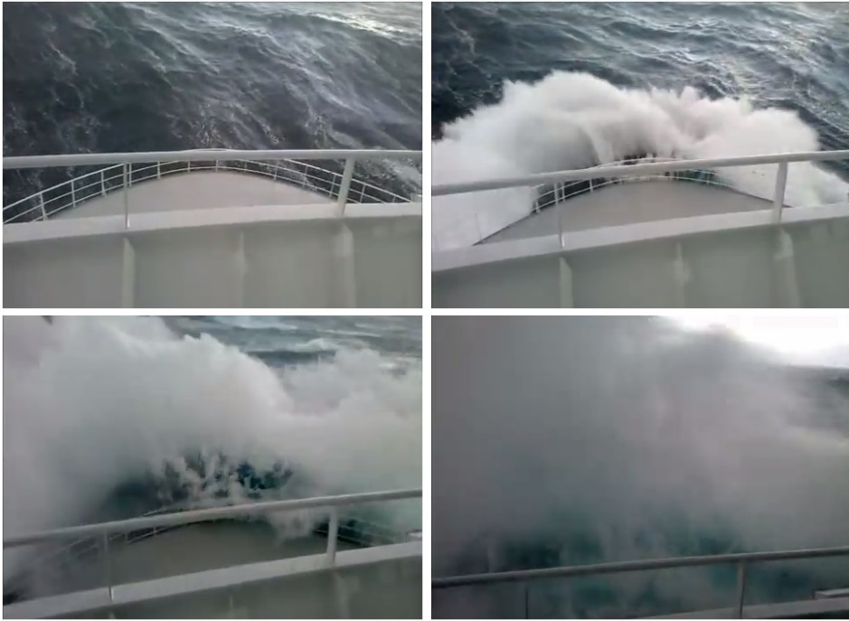
Figure 5.16: Bow slamming on Far Seeker (Leikarnes, 2011) – a platform supply vessel of the same UT 751 E design as studied in this chapter
