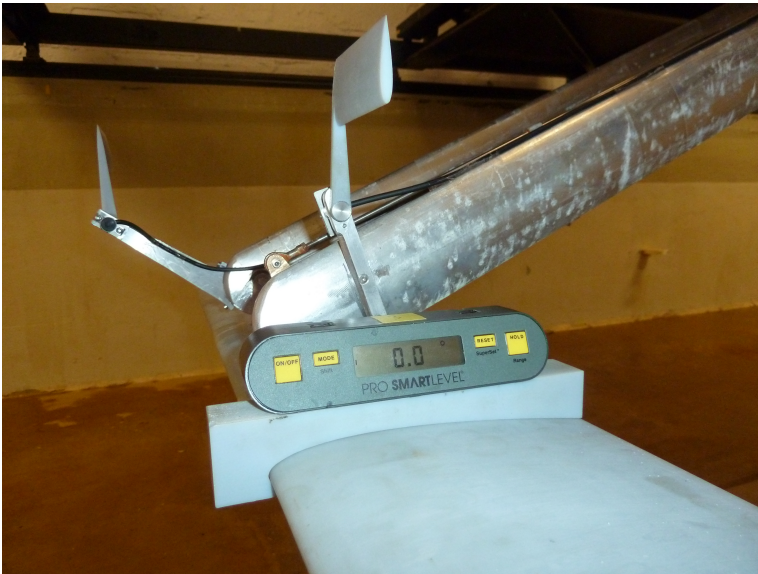
Figure B.2: Calibrating the foil pitch using a digital protractor. The digital protractor was placed on top of a removable part, fitting perfectly to the foil shape.
