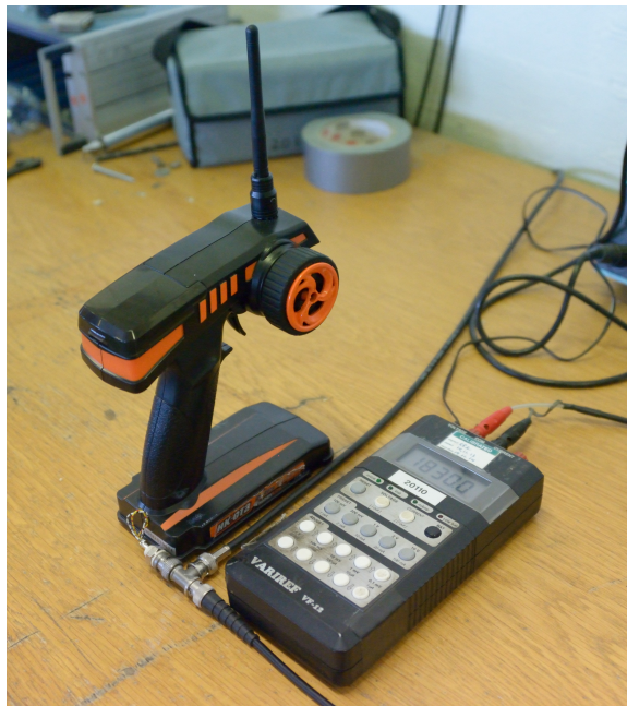
Figure 7.12: The remote control of the free-running ship model, with the throttle controlled by an external power source
