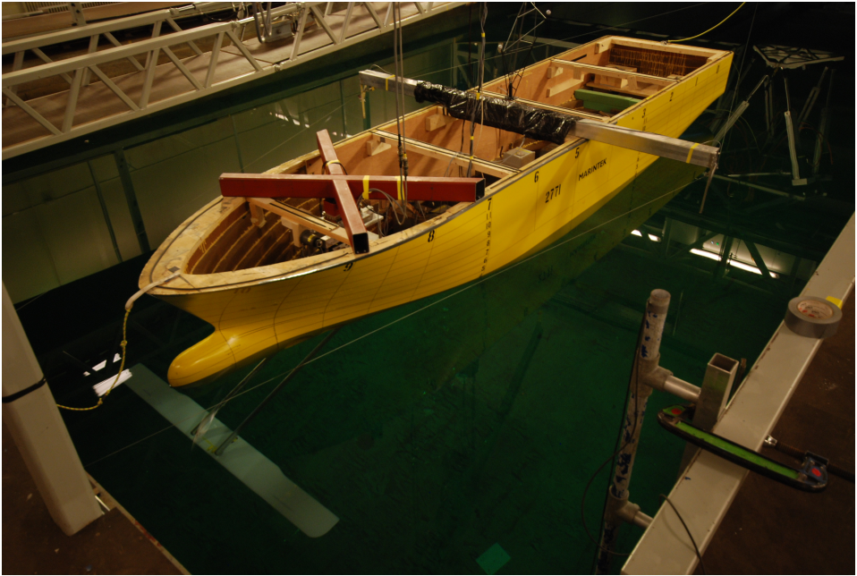
Figure 5.3: The setup in the March 2012 towing tank test
