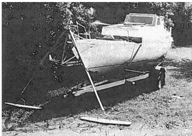
Figure 1.9: The bow of the 7.5 m hull used in tests on Wave Control Company's "foilpropeller" (Anon., 1983)
