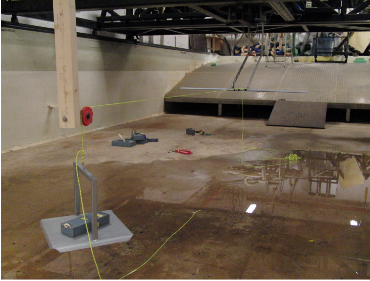
Figure B.1: Calibrating the force transducers using a rope, a pulley, and weights
