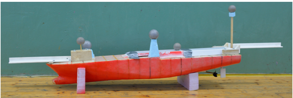
Figure 7.9: The free-running ship model on land, showing the front and back rail which the longer strut could be mounted on and the grey motion tracking balls. The front rail is bent up to avoid hitting the water.
