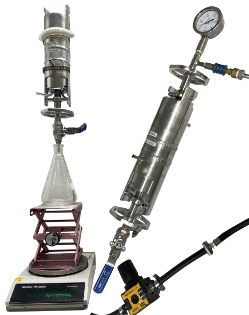
Figure 6: 0.35L BHS Sonthofen pressure filtration setup used for real process solution experiments.
