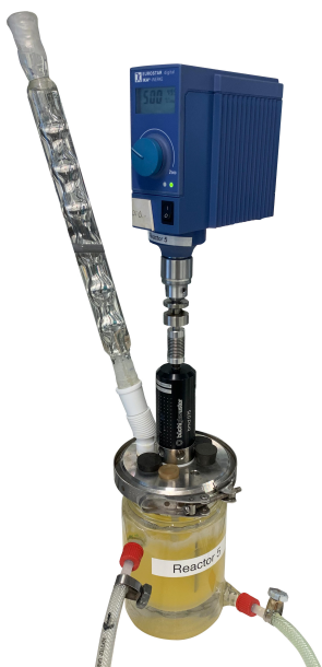
Figure 3: Batch reactor setup used in the synthetic solution experiments.
