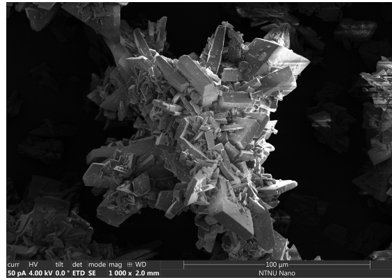
Figure I.33: SEM image of final crystals from continuous addition of the acid, in the synthetic system.
