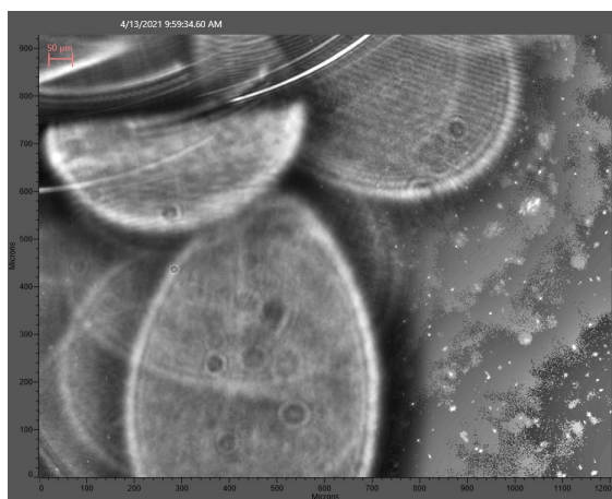
Figure L.52: Crystals were observed after 10-13min of the continuous addition of the acid experiment at 20°C (RPS).
