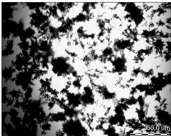
Figure 20: LM image of crystals from half way of the acid addition in continuous addition of the acid, in the synthetic system.
