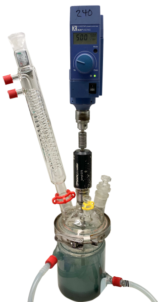
Figure 5: Batch reactor setup used in the real process solution experiments.
