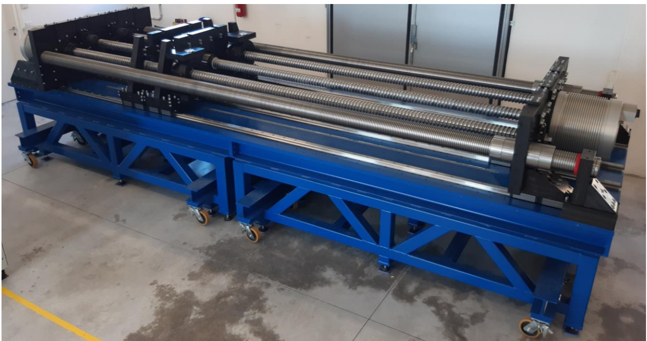
Fig. 14. HIL test rig mechanical assembly.
