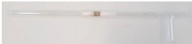
Figure 3.1: The quartz glass plug-flow reactor loaded with 50 mg of catalyst mixed with 150 mg of cordierite.
