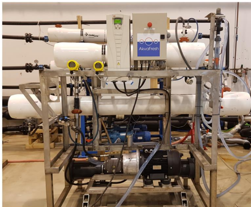
Figure 4.1 Picture of the same type of NF membrane installed at Sunndalsøra. (Picture provided by Akvafresh)
