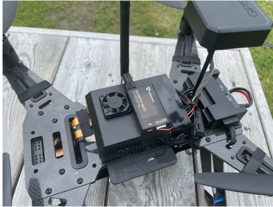
Figure 5.4: Telemetry radio is attached on top of a drone
