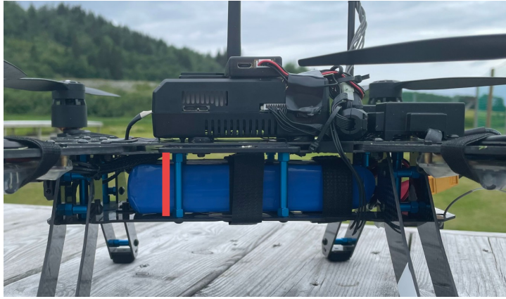
Figure 5.7: Battery position after adjustment
