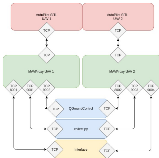
Figure B.1: Architecture for multi-vehicles experiment, two drones
