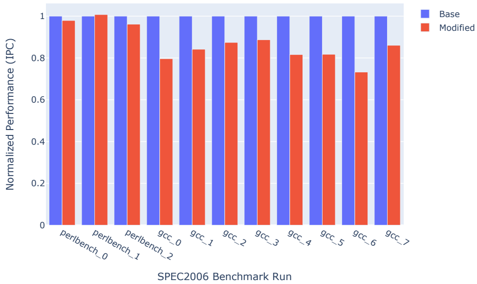
Figure 4.6: The instructions per cycle normalized to the baseline of the unmodified BOOM. perlbench and gcc are shown together.
