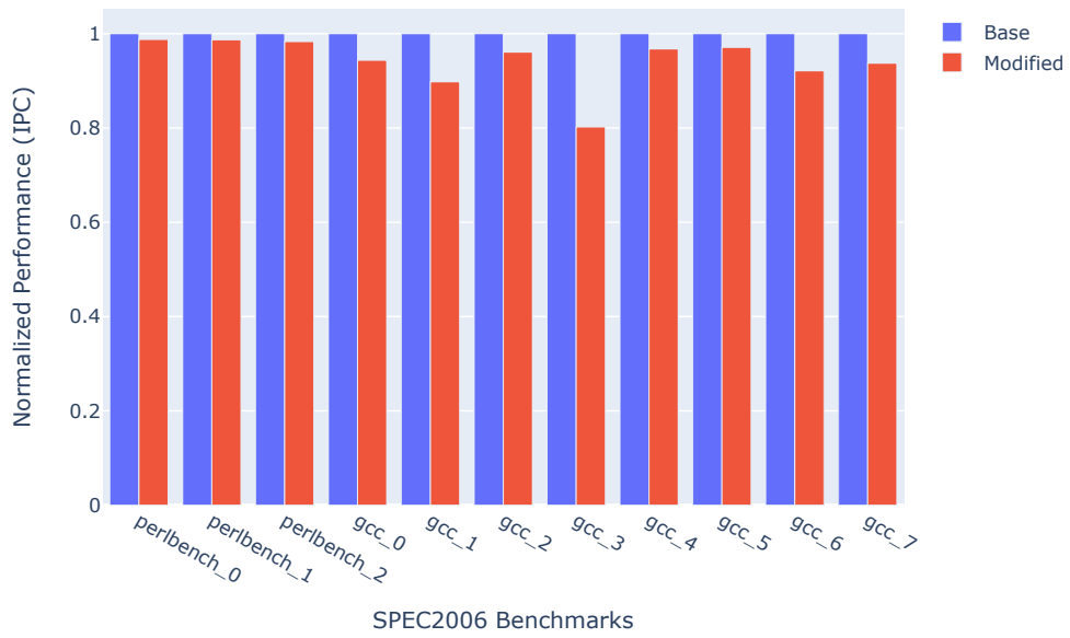
Figure 4.8: The instructions per cycle normalized to the baseline of the unmodified gem5 implementation using the O3 CPU. perlbench and gcc are shown together.
