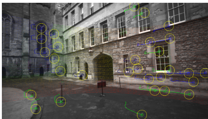
Figure 4.3: A visualization of data produced by the visual frontend showing tracked features and the LiDAR point cloud projected into the image. Features with depth are colored in blue, features without depth in green and yellow circles indicate IMU-propagated reprojection predictions from the backend.
