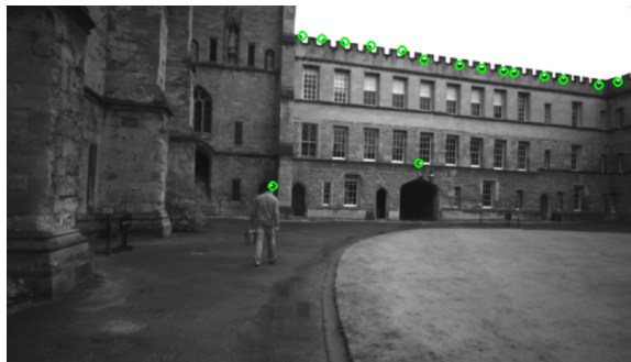
Figure 4.4: An example image taken from the Newer College dataset [39] where some Shi-Tomasi features are vastly stronger than others. In this case, the over-exposed sky along with the rectangular merlons cause nearly perfect corners with much higher quality scores than other feature candidates in the image.
