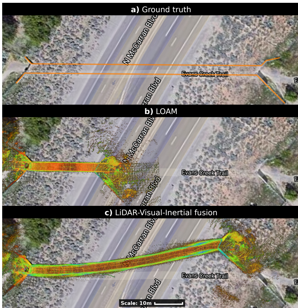
Figure 5.22: Qualitative results of running our system on the San Rafael tunnel dataset overlaid on Google Maps. The map of the tunnel produced by LOAM is much shorter than the ground truth, due to the geometric self-similarity of the tunnel. Our LiDAR-visual-inertial fusion gets comparatively closer to the real length, but also struggles in the middle of the sequence due to low landmark counts, and hence produces a geometrically inconsistent result.
