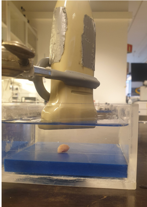
Figure 5.2: Experimental setup. The transducer is kept stable approximately 20 mm above center of the object to be imaged. Here tumor F is placed in the NaCl solution at 23 °C ready to be measured.
