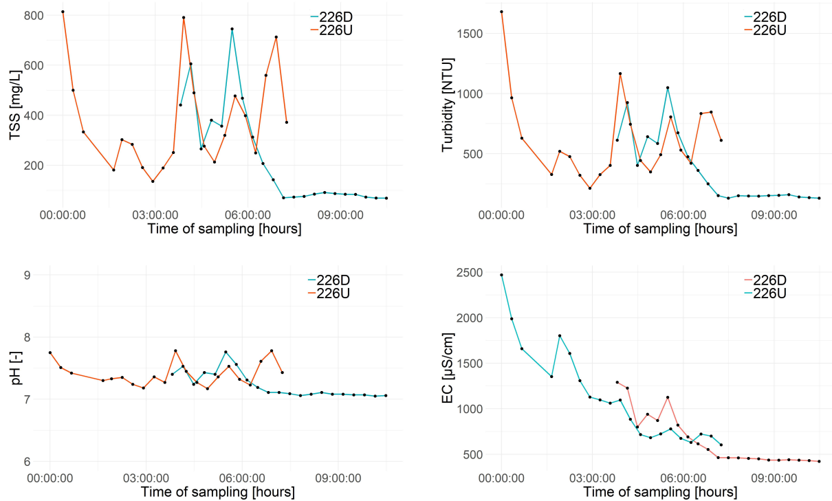
Results of lab analyses for TSS, Turbidity, pH and EC for the 25 th of February event. In the legend 226D represent the downstream and 226U the upstream flow.
