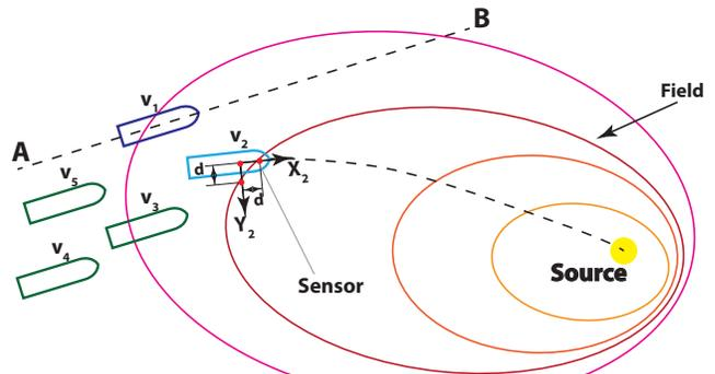
Fig. 1. Exchange of the leadership, the agent  $v_1$  is the initial leader, the agent  $v_2$  is the active follower, the red dots are the sensors
