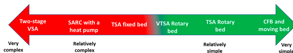
Figure 18. A simplistic illustration of the extent of complexity of the operating strategy of the different reactor configurations and operating mode.
