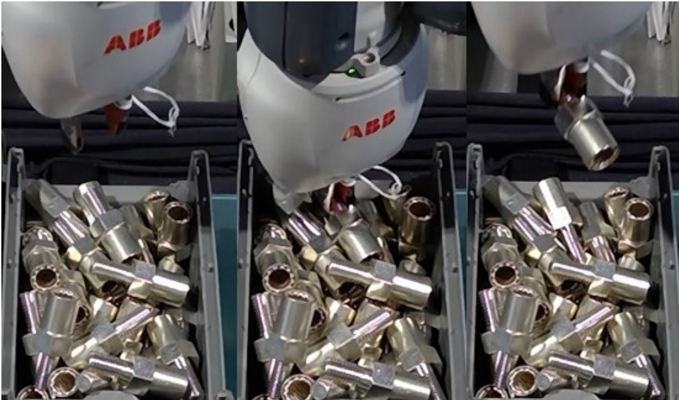
Figure 6.23.: Picking LFC at the threaded end. left) approach above pick, middle) gripping, right) picking the part
