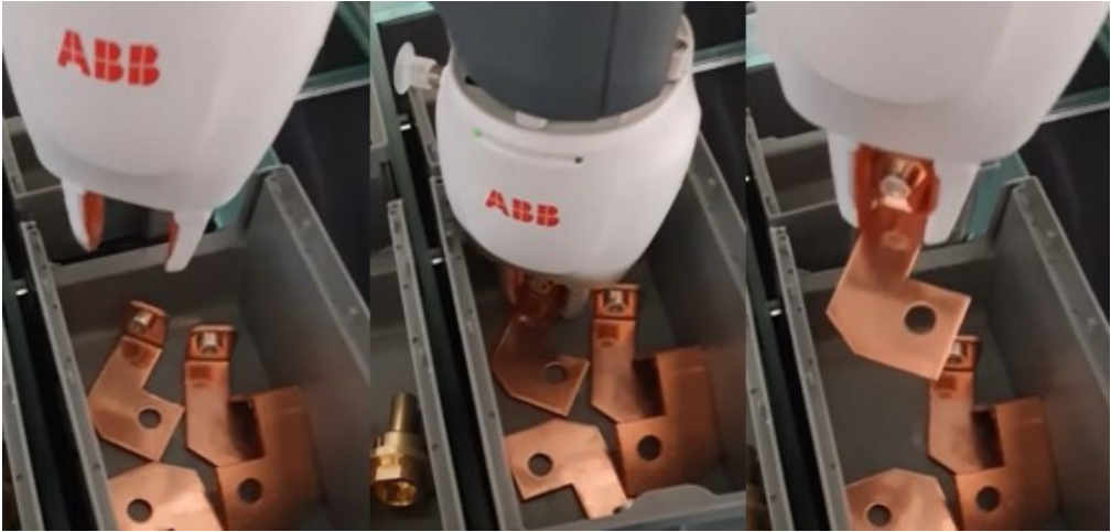
Figure 6.26.: Picking the large lask by the rules described in scenario 2. left) approach above pick, middle) gripping, right) picking the part
