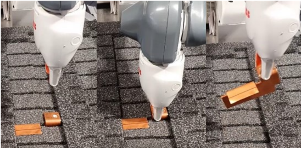
Figure 6.27.: Picking the elongated lask from the foam cutout. left) approach above pick, middle) gripping, right) picking the part
