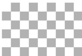
Figure 5.6.: Zivid recommended calibration object; gray/white checkerboard
