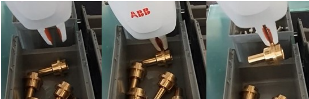
Figure 6.25.: Picking brass connector by the outer ring. left) approach above pick, middle) gripping, right) picking the part
