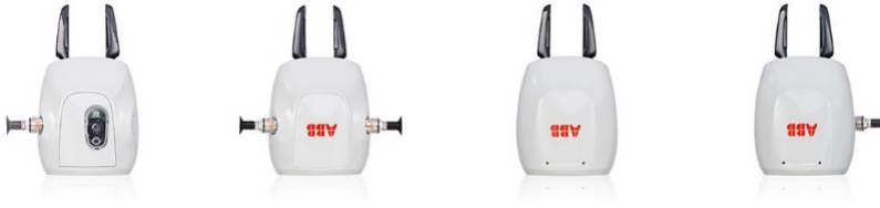
Figure 3.3.: YuMi Smart gripper configuration
