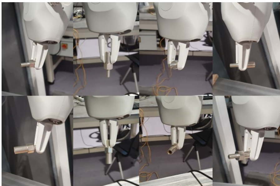
Figure 5.21.: Test of grip on various object poses of the female connector
