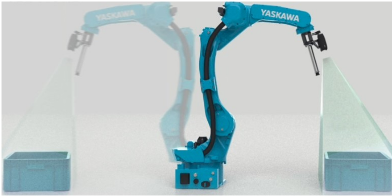
Figure 7.3.: Benefits of eye-on-hand configuration, robot reach defines workspace and the camera can be moved to the optimal position [95]
