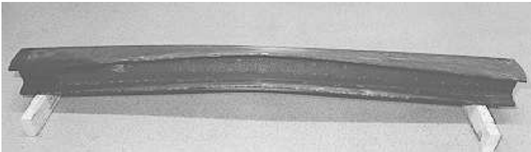
Figure B.9: Test specimen H-8-NMT, HEB 140 tested in axial load, bending and nonuniform torsion.
