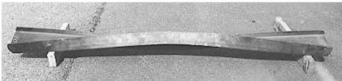
Figure B.8: Test specimen I-9-NT, IPE 160 tested in axial load and nonuniform torsion.
