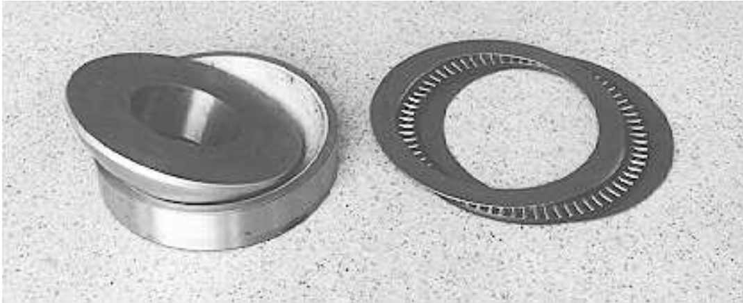
Figure B.3: Spherical thrust bearing (bending moment "hinge") and plane thrust bearing (torsional moment "hinge").
