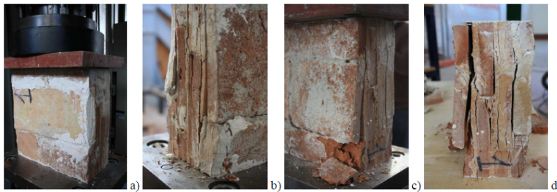
Figure 59: Samples: a)before the test; b,c)during the test d)at the end of the test
