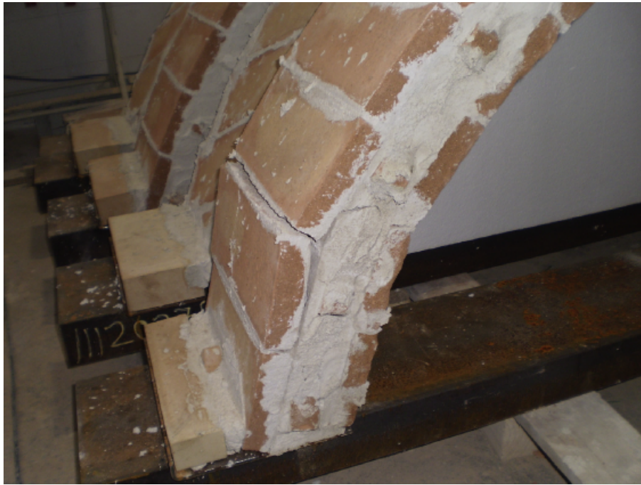
Figure 69: Shear sliding mechanism for arch TR.IT.01
