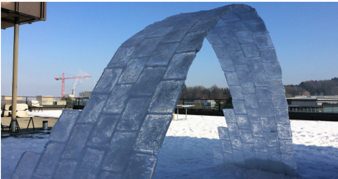
Figure 53: Ice tile vault
