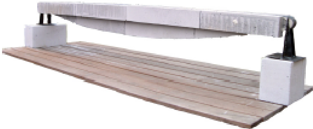
Figure 45: Hybrid masonry beam
