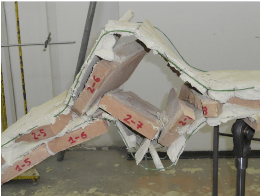
Figure 68: Ring separation and snap-through buckling; a) arch TR.IT.02; b) arch TR.OT.03
