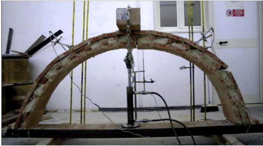
Figure 67: Arch displacement mechanism(arch TR.UT.01)
