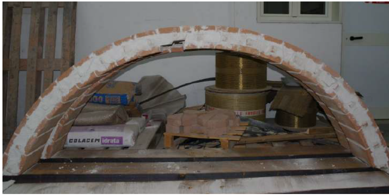
Figure 70: 4-hinges failure mechanisms
