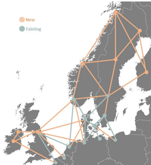
Figure 22: New lines and nodes (orange) was added in the input files to better fit the 2040 scenarios. All TYNDP 2020 scenarios had the same grid structure. The new lines and nodes are according to TYNDP 2020. The blue nodes and lines was already included in the 2014 data set. Created by the author.
