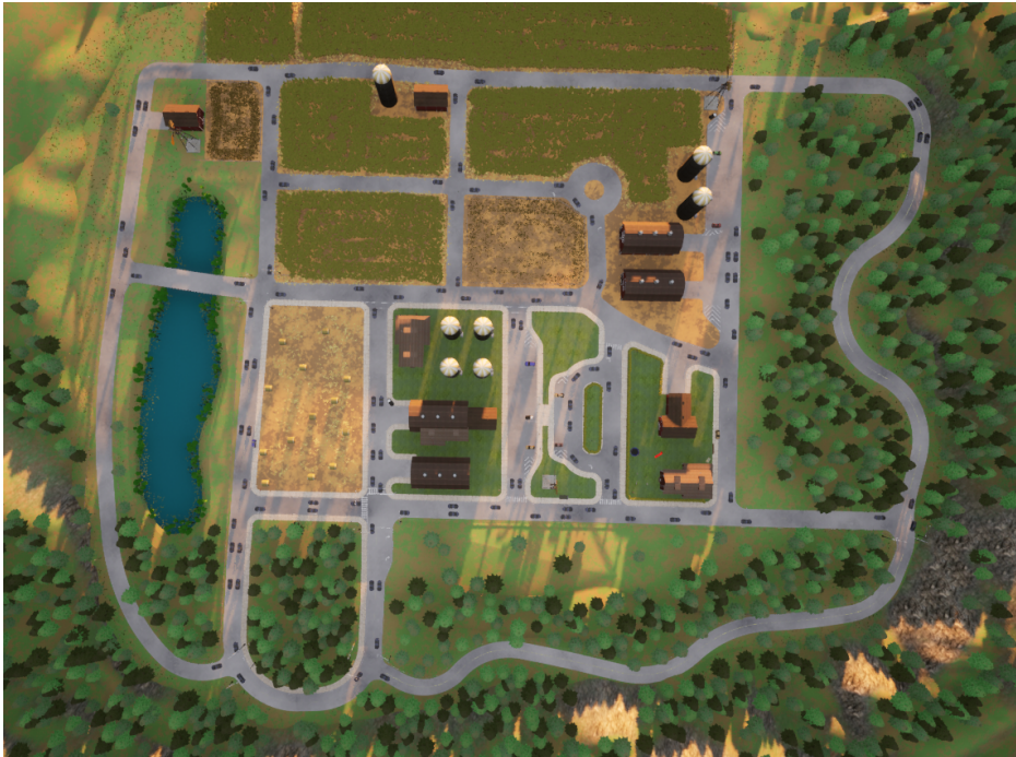
Figure 3.10: A birds-eye view of the Town07 map in Carla. The spawnpoints have been visualized by spawning a black car at each one. The lane-following parts can be seen in the west, south and east outskirts of the map.
