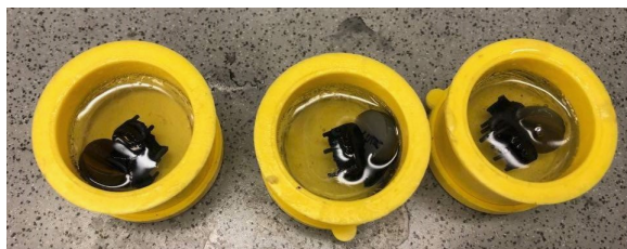
Figure 3.8: Cross-sectional analysis to estimate coating thicknesses of gold-sputtered coatings were not possible to perform as the cross-sectional samples tilted during the curing of the epoxy casting material.
