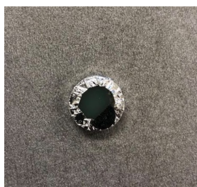
Figure 3.10: A four layer DGEBA coated sample after being sputter coated with gold and covered in aluminum film and conductive tape prior to surface topography analysis in SEM.
