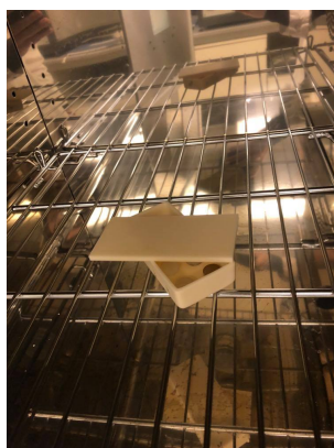
Figure 3.6: Coated PE-substrates placed in an alumina box with the lid placed partially off.
