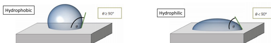
Figure 2.11: Liquid drop on a substance having a hydrophobic surface and hydrophilic surface. Figure adapted from [149].
