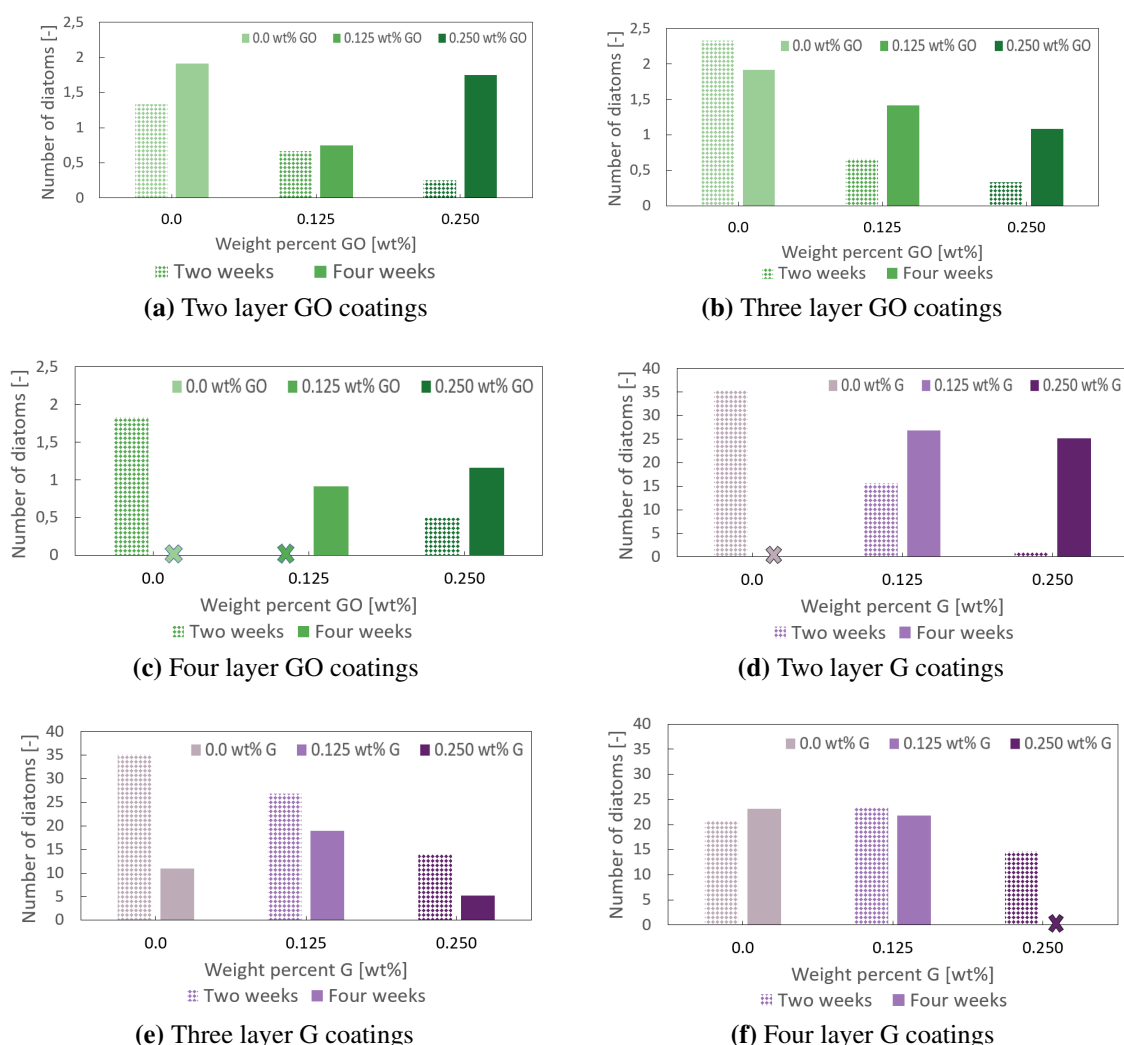
Figure 4.20: Number of diatoms measured on 0.0 - 0.250 wt% GO coatings with a) two, b) three and c) four coating layers and 0.0 - 0.250 wt% G coatings with d) two, e) three and f) four coatings layers. Diatom growth after submersion for two weeks (dotted bars) and four weeks (continuous bars) are shown. Unrepresentative data points are removed and marked with a cross.
