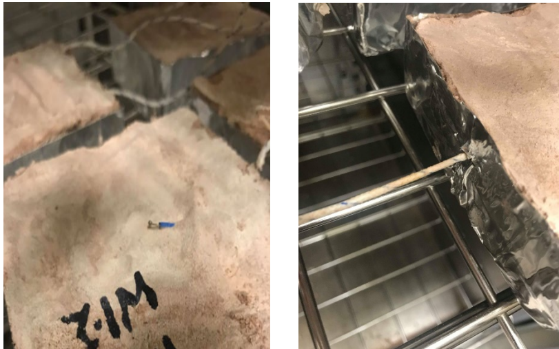
Figure 5. (L) Thermocouple cast on the surface of mortar (R) Thermocouple cast 15mm from surface of earth mortar composite.
