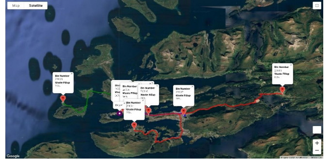
Figure 8. Optimized routes via CVRP with minimum duration for V_N and N = 0,1,2
