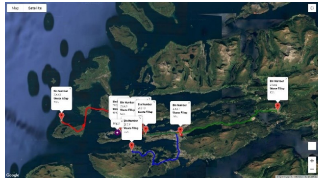
Figure 6. Optimized routes via VRP with minimum duration for V_N and N = 0,1,2
