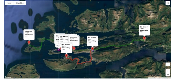
Figure 9. Optimized routes via CVRP with minimum distance for V_N and N = 0,1,2
