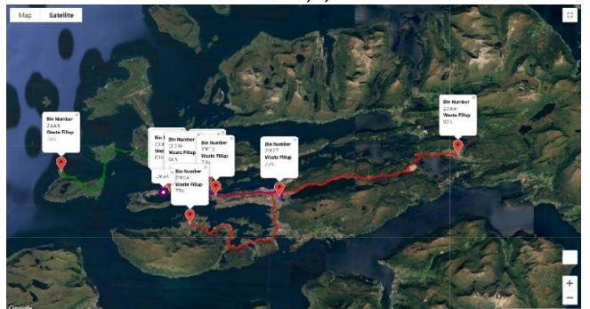
Figure 7. Optimized routes via VRP with minimum distance for V_N and N = 0,1,2
