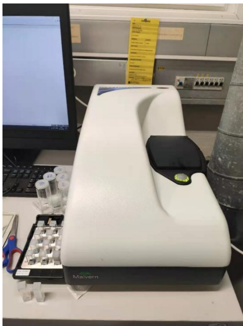
Fig. 34: Dynamic light scattering device is Zetasizer ZS90 from Malvern Panalytical.
