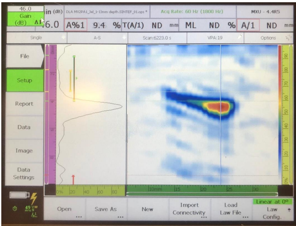
Figure 32, The final PAUT after the test was terminated. This photo is provided by Hans Lange from SINTEF.
