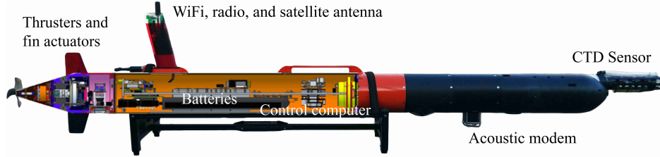
FIG 9. The commercially available Light Autonomous Underwater Vehicle (LAUV) platform for upper water-column exploration used in our experiments.
