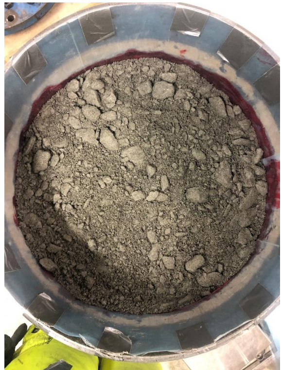
Figure 0.41 TBM 4, fourth layer, not compacted
