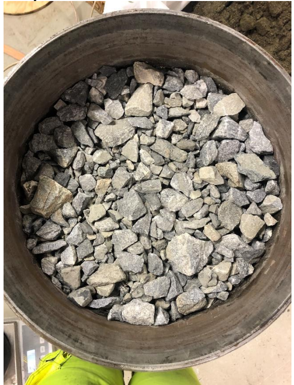
Figure 0.47 CR 1, fourth layer, compacted
