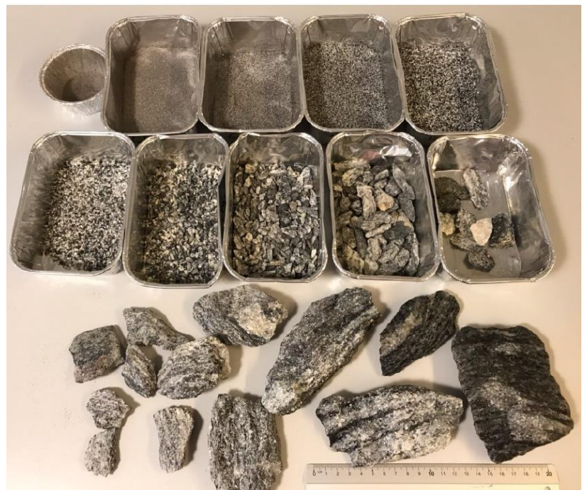
Figure 2.5 Sieved and washed TBM spoil from the Follo Line Project (NGI, 2019a)
