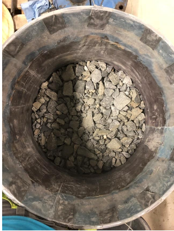
Figure 0.61 CR 3, second layer, compacted
