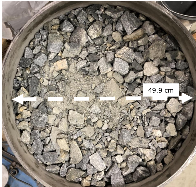
Figure 3.15 Crushed rock placed in oedometer cell
