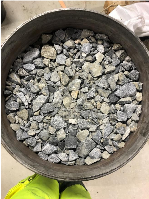
Figure 0.51 CR 1, fifth layer, compacted
