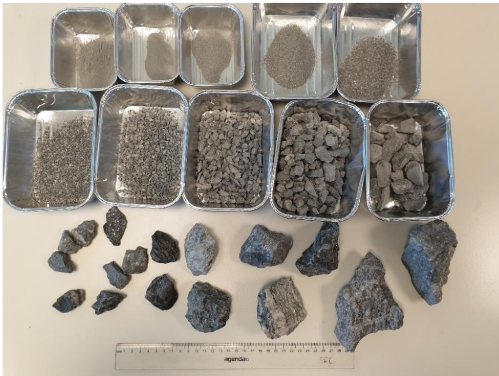
Figure 2.23 24 Sieved and washed D&B spoil from Akershusstranda (NGI, 2020)
