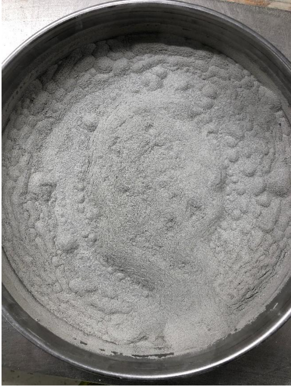
Figure 0.34 TBM 3, sieving analysis, 63 μm
