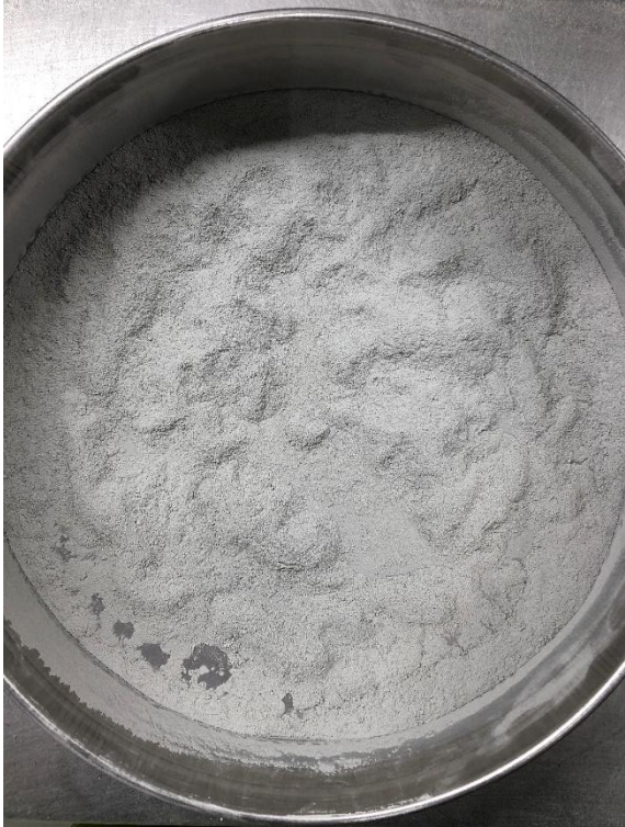
Figure 0.38 TBM 3, sieving analysis, <63 \mu\text{m}
