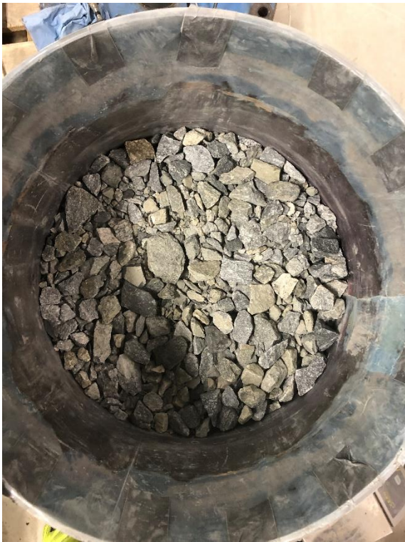
Figure 0.60 CR 3, third layer, compacted
