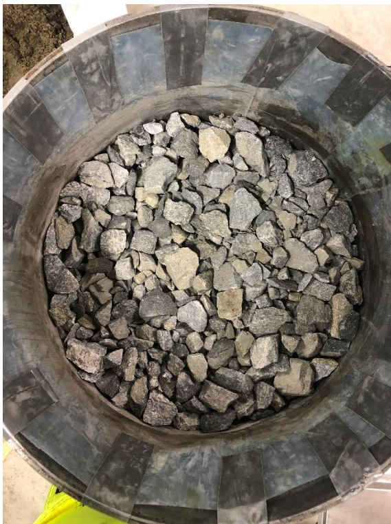
Figure 0.48 CR 1, third layer, compacted
