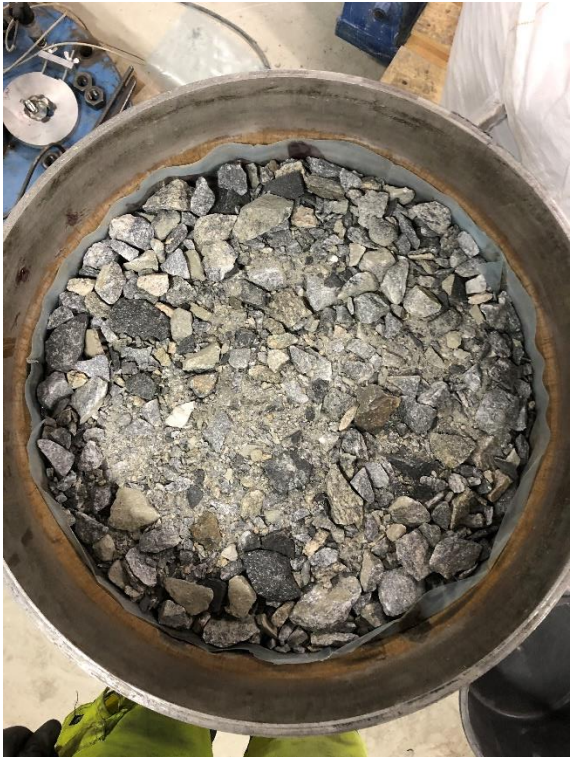
Figure 0.53 CR 2, fourth layer, compacted
