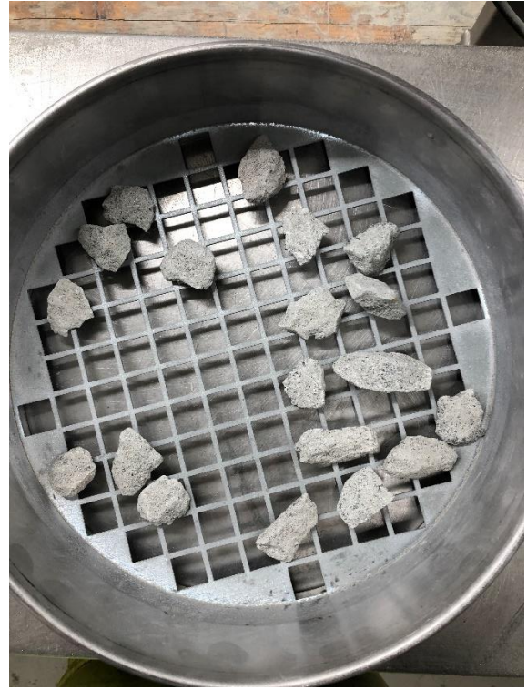
Figure 0.28 TBM 3, sieving analysis, 19 mm
