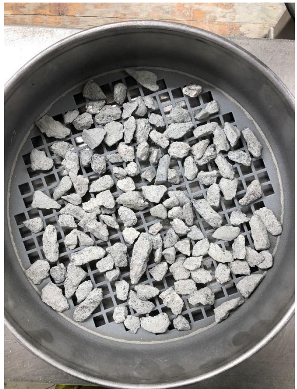
Figure 0.26 TBM 3, sieving analysis, 11.2 mm
