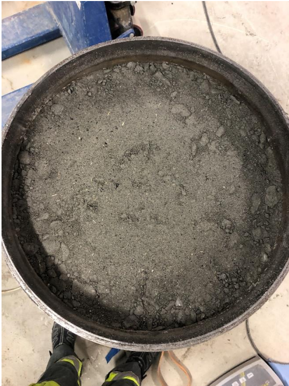
Figure 0.11 TBM 1, fifth layer, compacted
