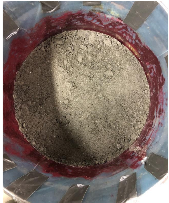
Figure 0.8 TBM 1, third layer, compacted
