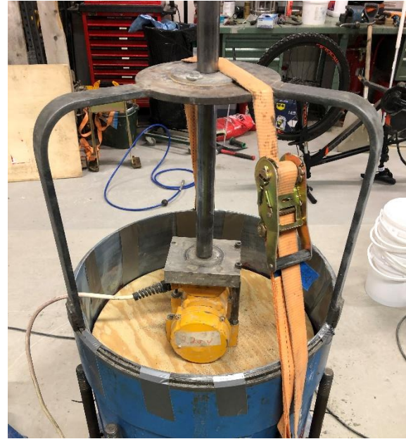
Figure 3.1 Compaction of material
