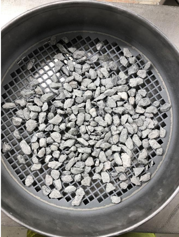
Figure 0.32 TBM 3, sieving analysis, 8 mm
