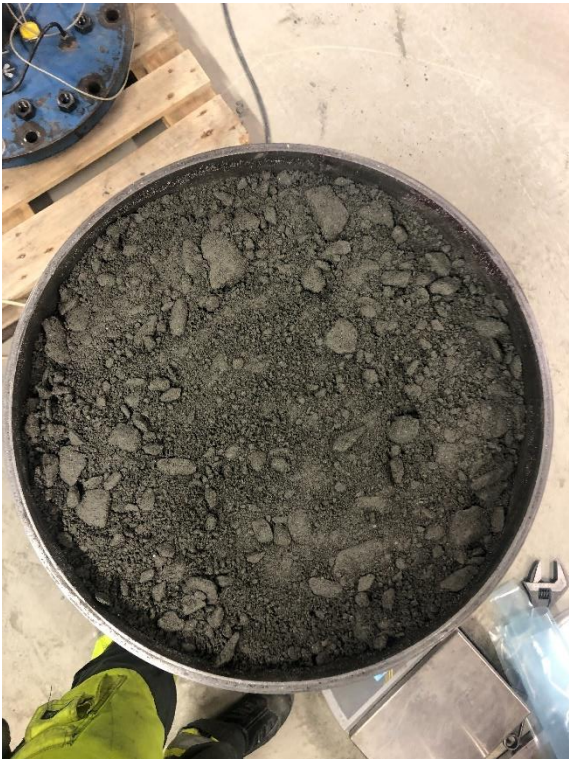
Figure 0.43 TBM 4, sixth layer, compacted
