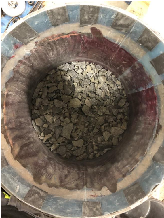
Figure 0.55 CR 2, first layer, compacted
