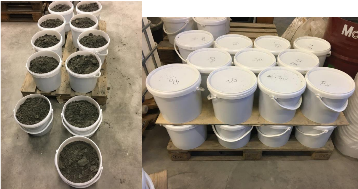
Figure 3.7 To the left: The content in the TBM spoil buckets. To the right: The amount of two tests. Pictures taken by KSR-Maskin.
