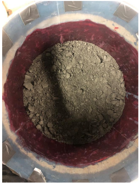
Figure 0.40 TBM 4, second layer, not compacted
