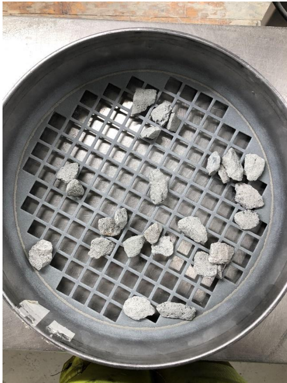
Figure 0.27 TBM 3, sieving analysis, 16 mm
