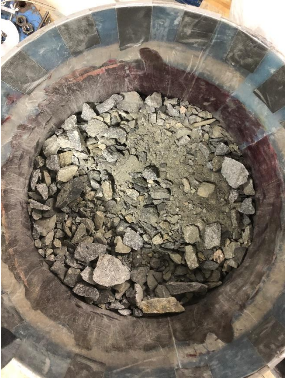
Figure 0.54 CR 2, second layer, not compacted
