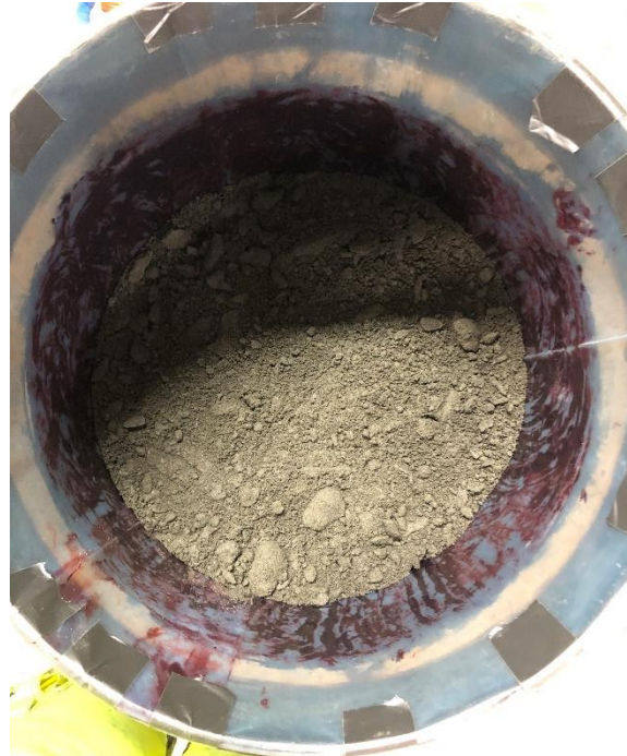
Figure 0.23 TBM 3, second layer, not compacted
