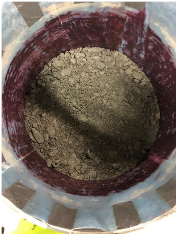
Figure 0.15 TBM 2, second layer, not compacted
