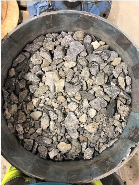
Figure 0.65 CR 3, fifth layer, compacted
