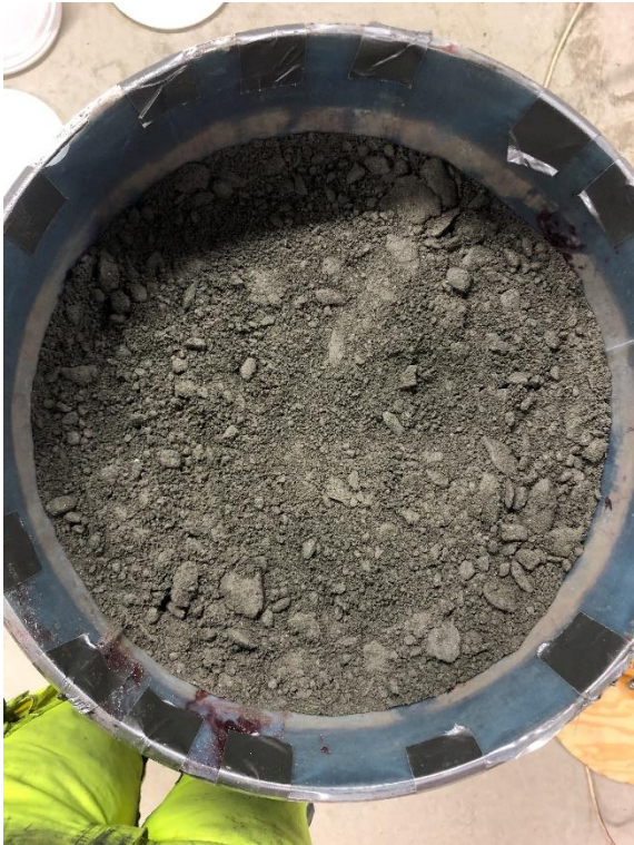
Figure 0.25 TBM 3, fifth layer, not compacted
