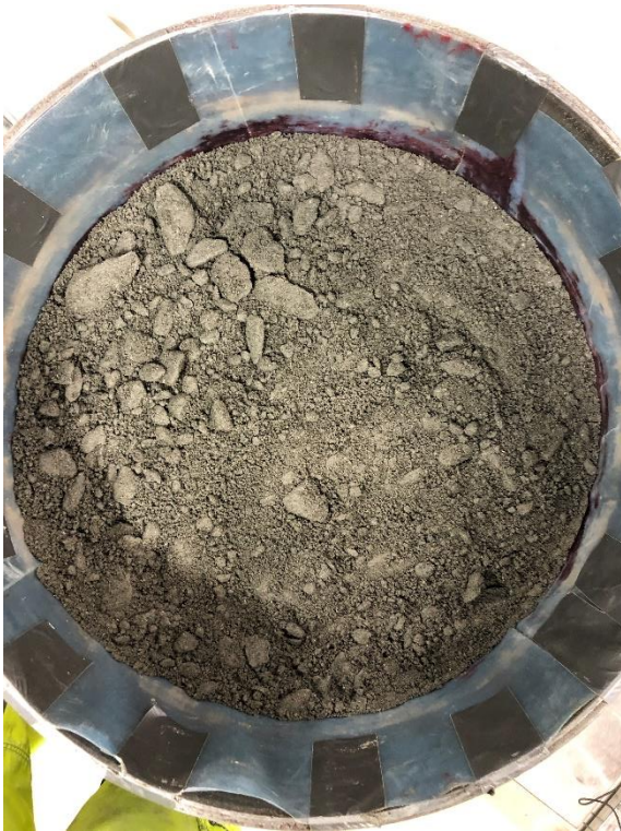
Figure 0.20 TBM 2, fourth layer, not compacted
