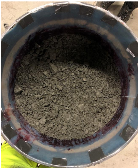
Figure 0.22 TBM 3, third layer, not compacted
