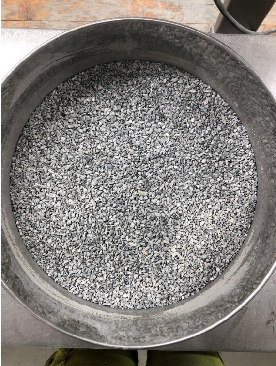
Figure 0.30 TBM 3, sieving analysis, 2 mm
