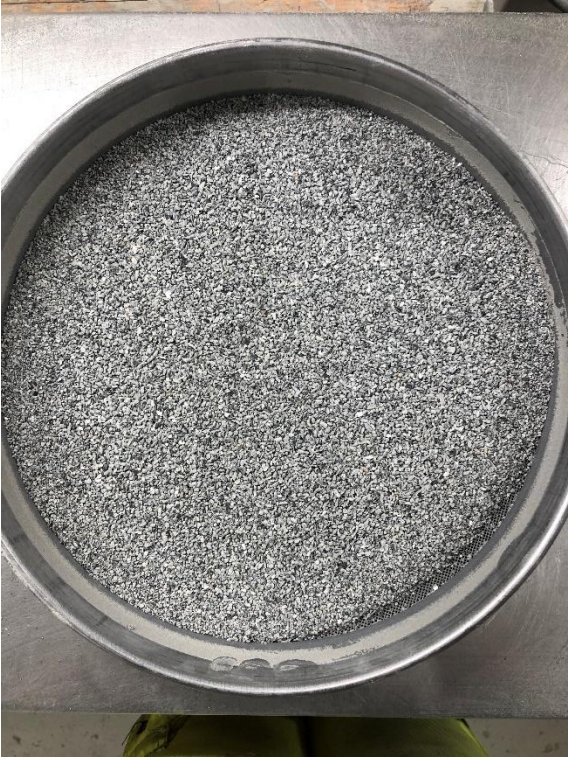
Figure 0.31 TBM 3, sieving analysis, 1 mm
