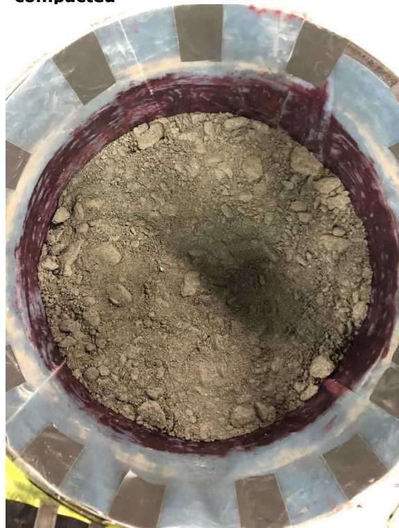
Figure 0.13 TBM 2, third layer, not compacted
