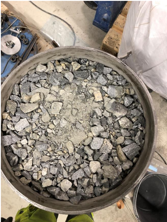
Figure 0.57 CR 2, sixth layer, compacted
