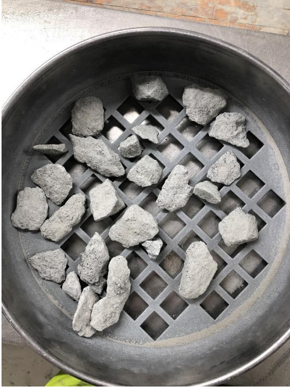
Figure 0.29 TBM 3, sieving analysis, 22.4 mm
