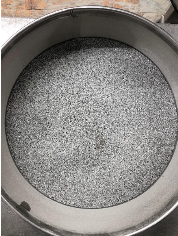
Figure 0.37 TBM 3, sieving analysis, 0.5 mm
