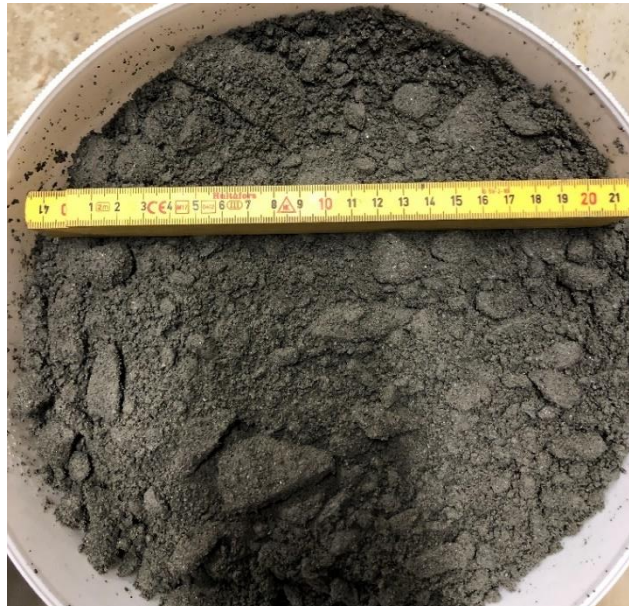
Figure 3.13 TBM spoil in the delivered buckets
