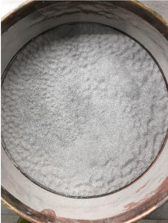
Figure 0.35 TBM 3, sieving analysis, 0.125 mm
