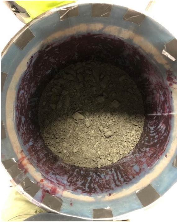
Figure 0.24 TBM 3, first layer, not compacted
