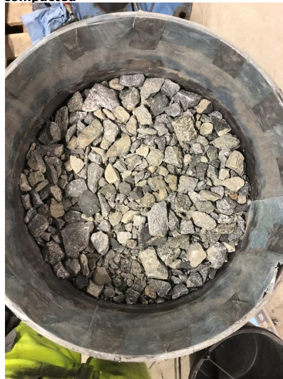
Figure 0.59 CR 3, fourth layer, not compacted
