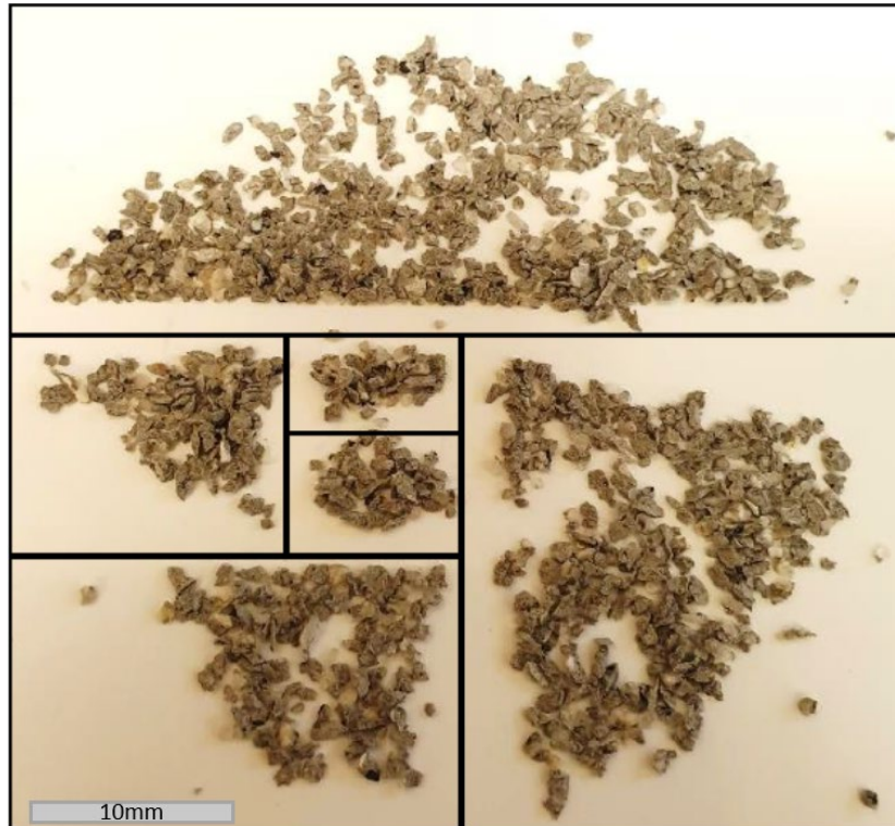
Figure 2 – Subdivision of scaled particles after sieving (salt frost test 040-330, 0-5 cy).
