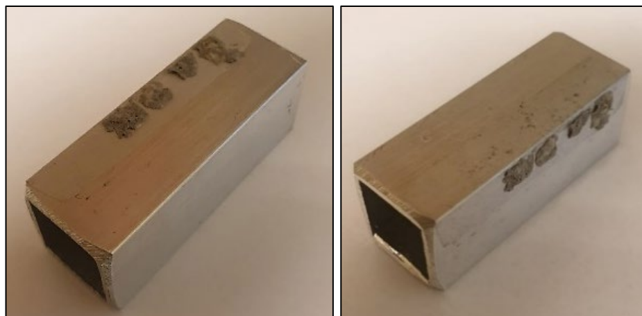
Figure 3 – Fixing of particles on 40 x 40 mm metal profile with double-sided tape for digital calliper calibration and measurement of Length ( L ), Width ( W ) and Thickness ( T )
