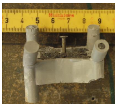
Figure 54: Representative plastic spacer removed from Beam B showing a nail in the middle with potential contact to the reinforcement steel
