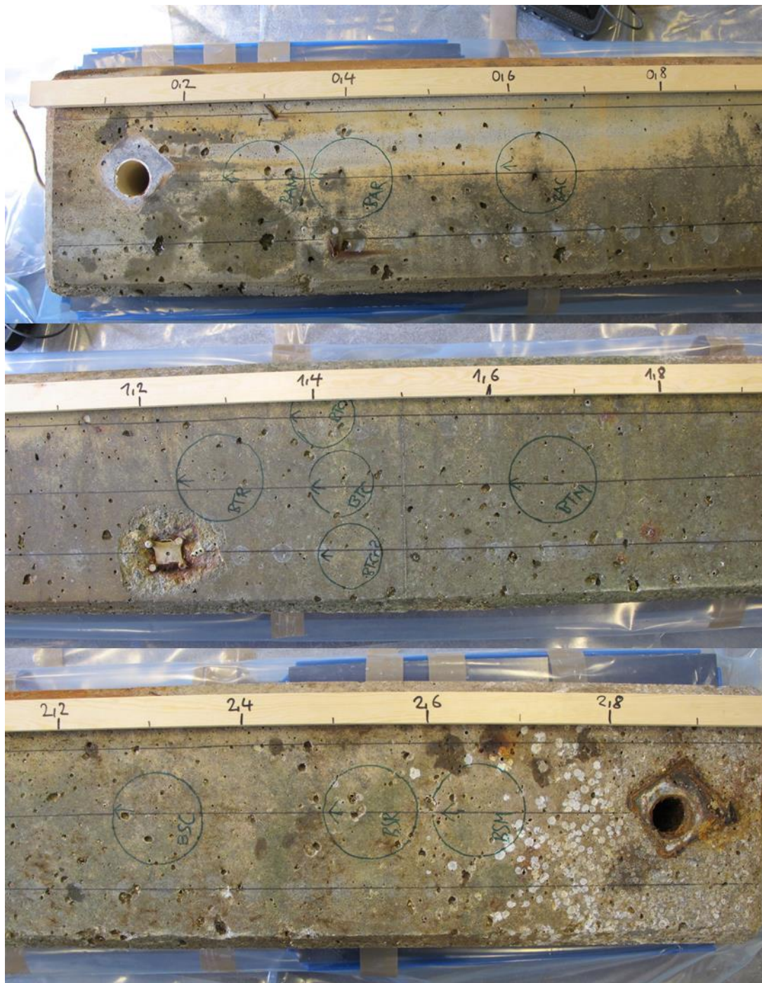
Figure 2: Location of concrete cores taken from Beam B, distance in meters (Photos: Eva Rodum)
