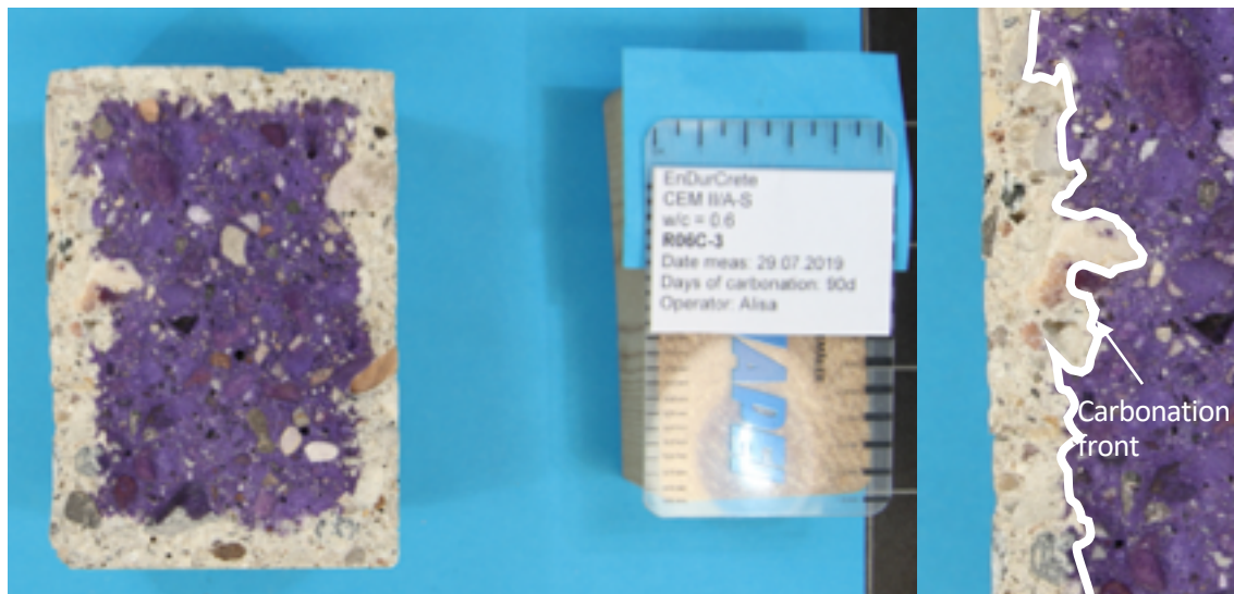
Figure 6 Example of cracked concrete sample sprayed with thymolphthalein solution (left) and detail of the carbonation front (right). Illustration: (Bjørndal, 2019)
