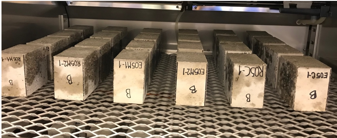
Figure 3 Sawn blocks ready for exposure in the carbonation chamber.
