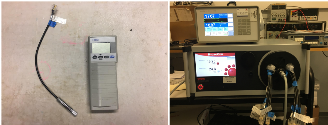
Figure 10 Left: HMP44 temperature and humidity probe and HMI41 indicator. Right: Calibration setup: MBW 473-RP2 (top) and Rotronic Hygrogen2(bottom) with the HMP44 sensors and the dew point mirror hygrometer probe from the MBW 773-RP2 (grey wire) inserted.
