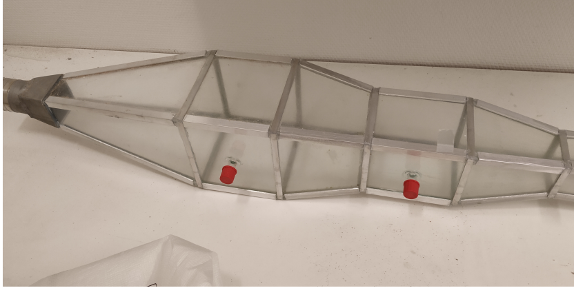
Figure 5.2: First version of the droplet generation section.
