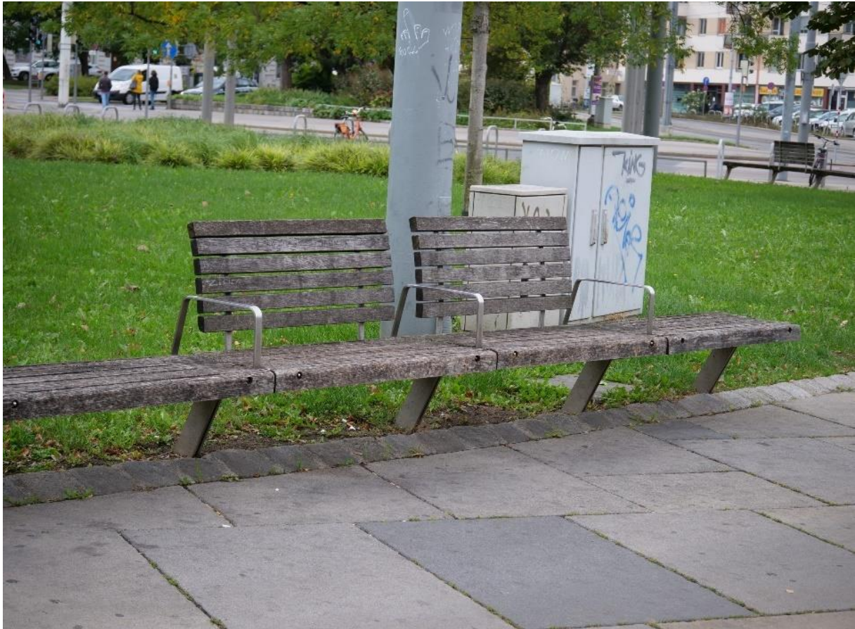
Figure 4: Armrests that should prevent people from sleeping - an example for deterrent design (Wölfl, 2019)
