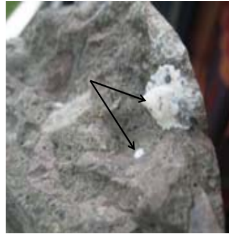
(b) Normal occurrence of ASR gel on structures
