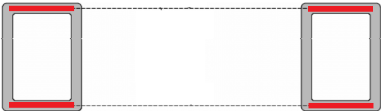
Figure 9.4: Placement of reinforcement in the flange
