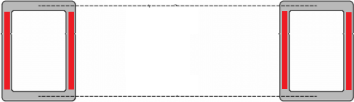
Figure 9.10: Placement of reinforcement in the web
