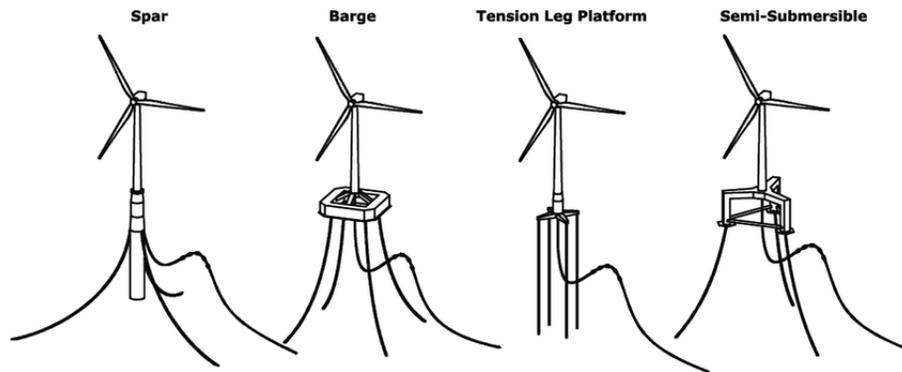
Figure 1: Substructures [40]
