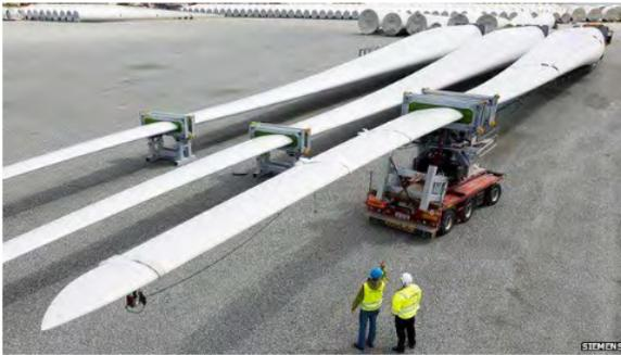
Transportation of blades can be similar to the transportation from quayside to storage area, with rolling special trucks, SPMT or crane from storage area to assembly area for hub and blades. The mounting of the blade to the hub requires a crane. Therefore, for logistic simplification, the blade will be transported with some sort of rolling transportation, enabling a crane in the assembly area to easily pick up the blade and start the mounting.
