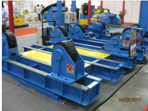
Figure 15: Pipe turning roll [37]
