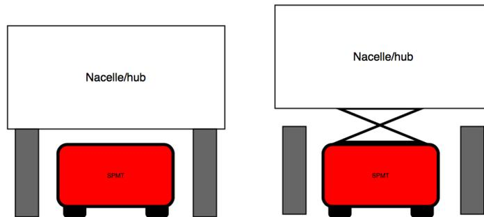
Figure 11: SPMT lifting nacelle/hub
