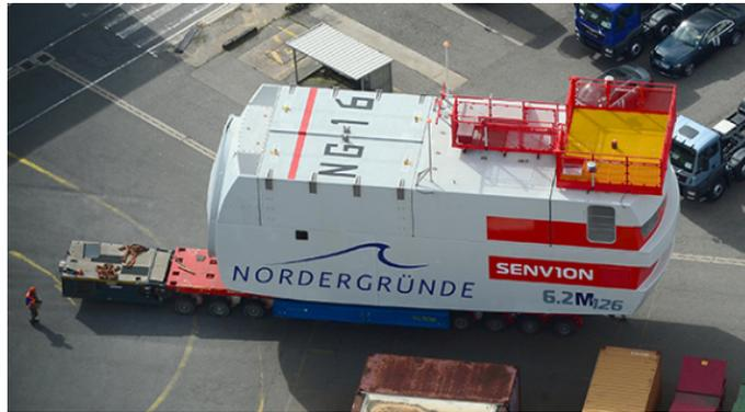
Figure 10: Nacelle on SPMT[12]
