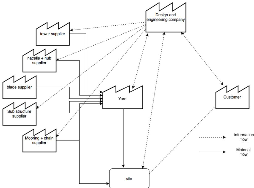
Figure 2: supply chain floating wind turbine
