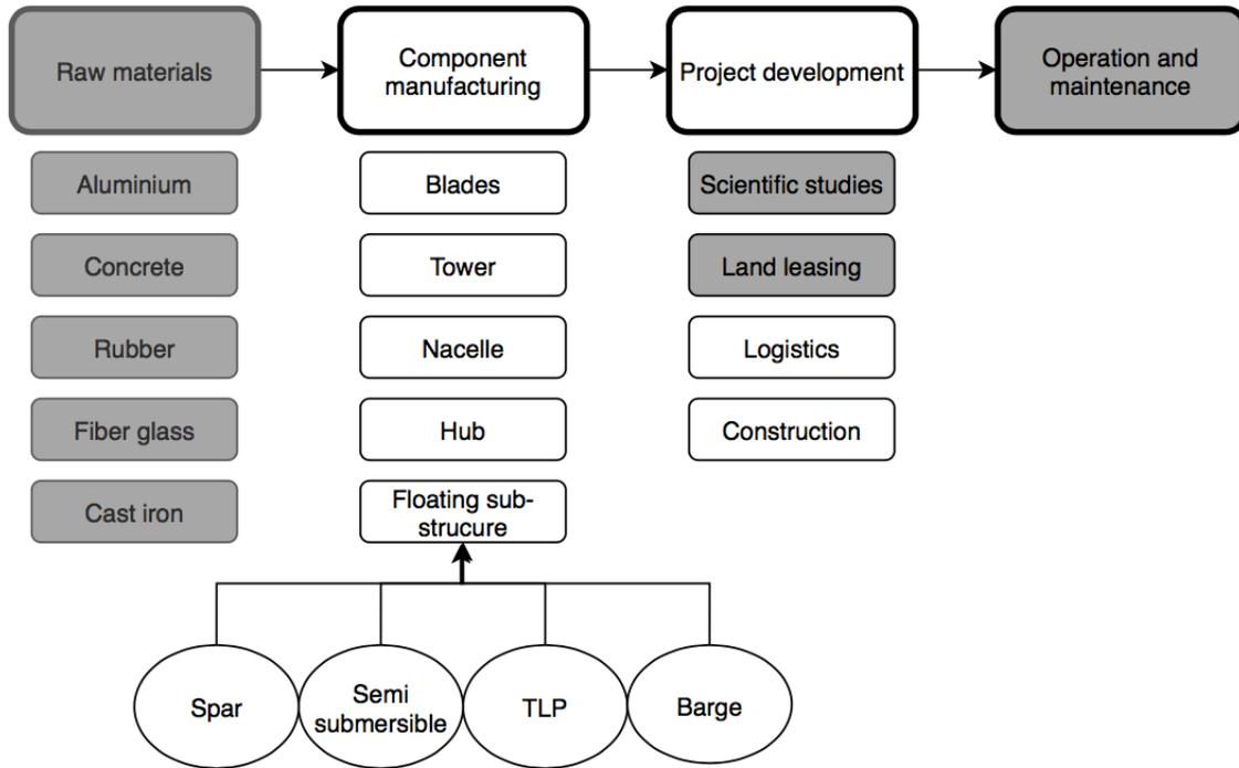
Figure 3: Simplified sketch of main actors in production of a floating wind turbine
