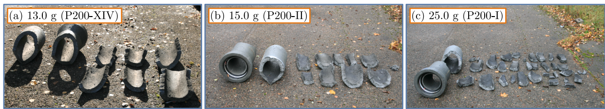
Fig. 6. Fragmented P200 pipes after testing with spherical C-4 charges detonated from position (i), for (a) 13.0 g, (b) 15.0 g, and (c) 25.0 g.
