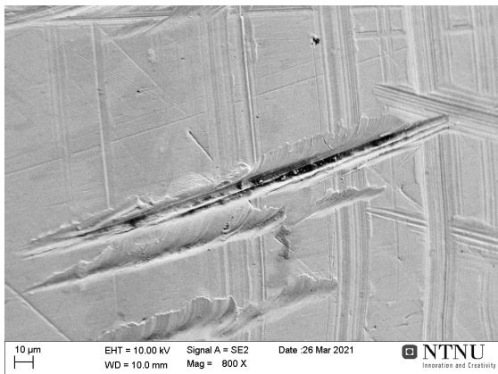
Figure 66: Prosthesis SS Scratch on the neck
