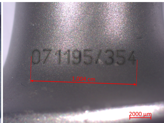
Figure 32: Prosthesis Co Markings on side 1 of the neck
