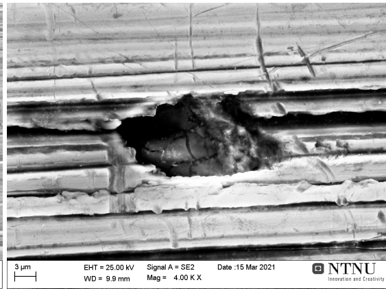
Figure 81: Prosthesis Co-o Sub surface particle
