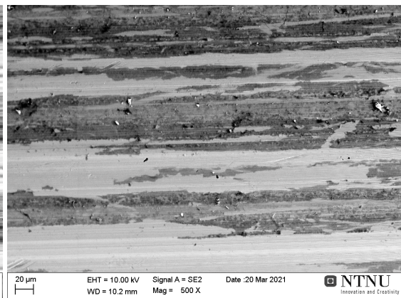
Figure 71: Prosthesis Co Flatter ridges with discoloration
