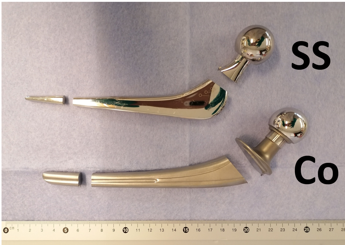
Figure 13: The cuts made prior to SEM
