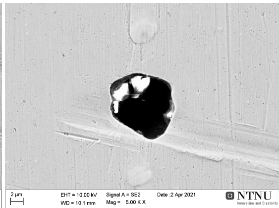
Figure 67: Prosthesis SS Pore on the stem
