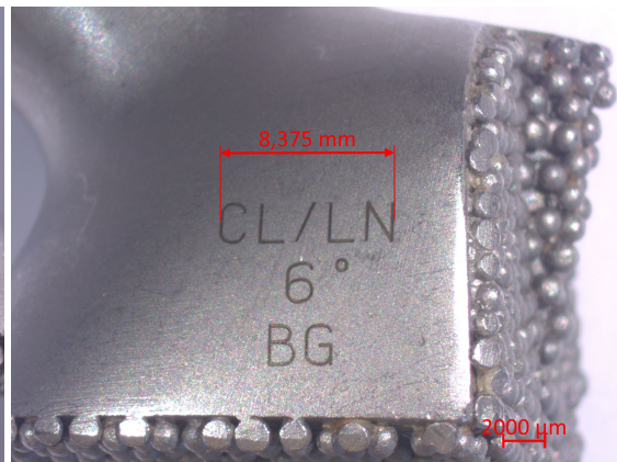
Figure 36: Prosthesis Co-o Markings on side 2 of the neck
