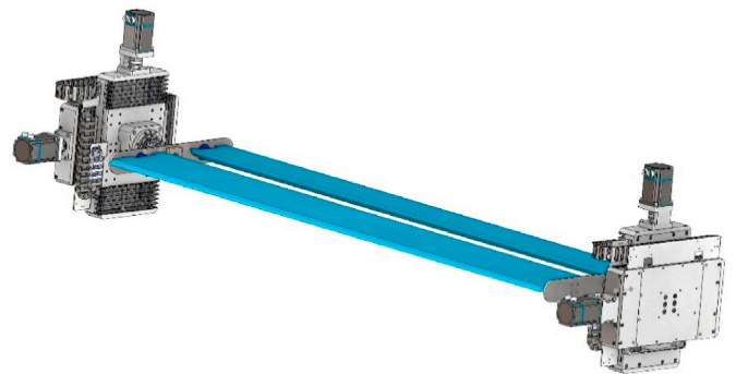
Fig. 4. Illustration of the test rig. Two actuators, one at each side of the wind tunnel, can force the section model to move in the horizontal, vertical and pitching directions.
