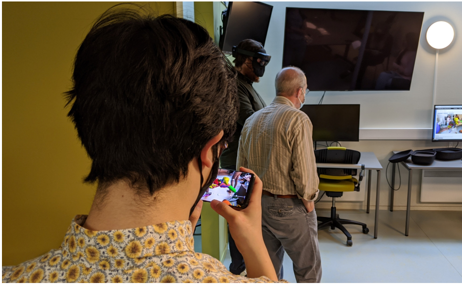
Figure 4.3: Networking allows the Android test user to see the same brain model as the HoloLens 2 user. The monitor on the background displays a live feed from the HoloLens device.
