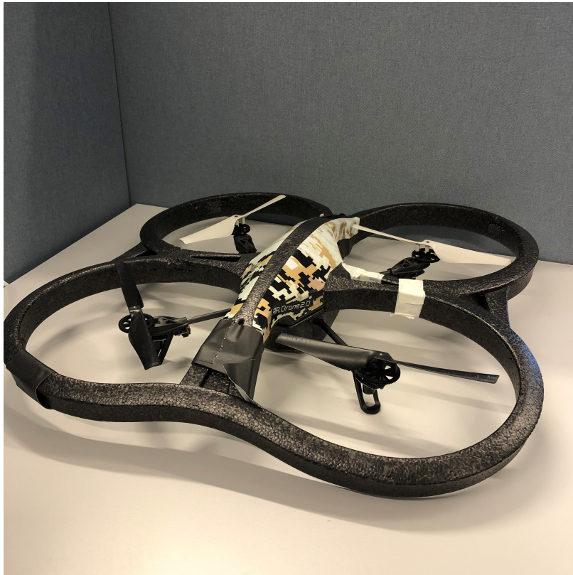
Figure 4.3: Picture of the AR parrot drone 2.0 used for experiments.
