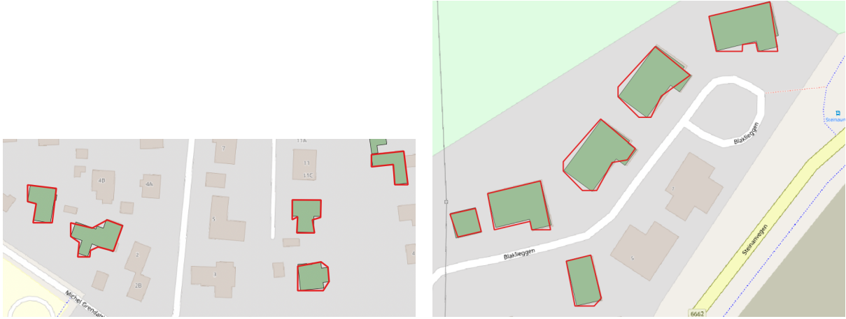
Figure 5.5: Predicted polygons from alpha-shape input presented with the ground truth polygons.
