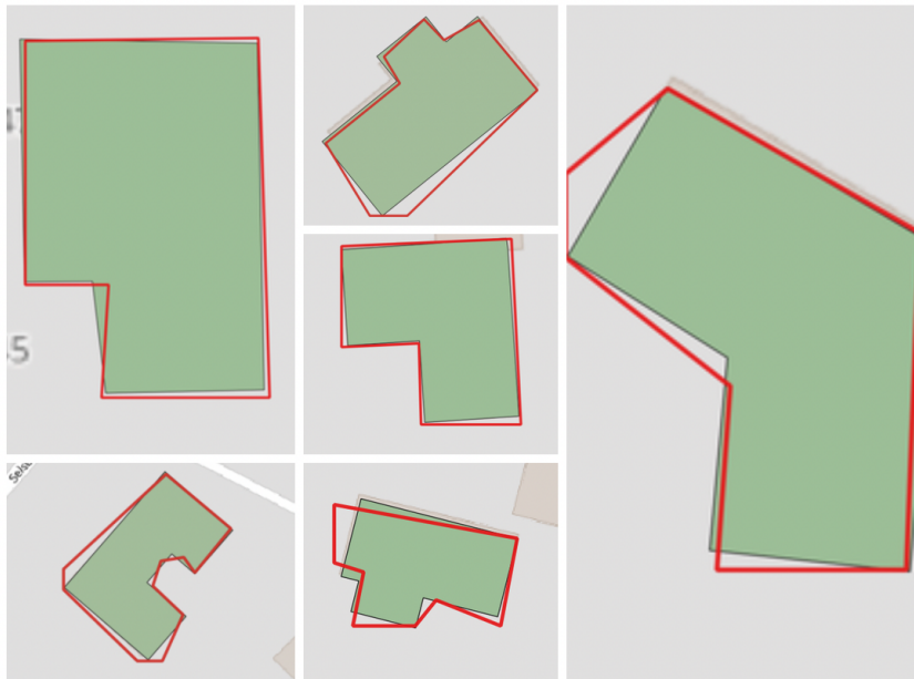
Figure 5.3: Close up of samples of polygons with different geometrical properties. Note the misalignment of edges.
