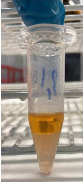
Figure 3.4 Picture of fluid collected after CTF extraction, the top phase is oil extract, and the lower phase is water based CTF extract in an Eppendorf tube.
