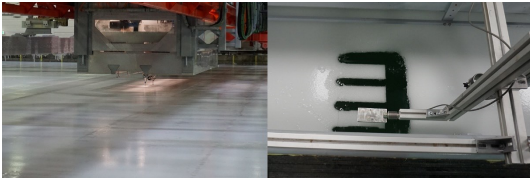
Fig. 3.14 Flexural strength measurements, cantilever beams
