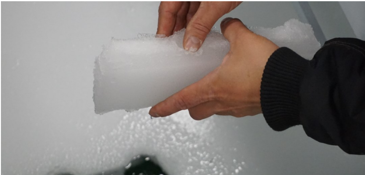
Fig. 3.5 Layering of the ice, strong top layer, weak bottom layer
