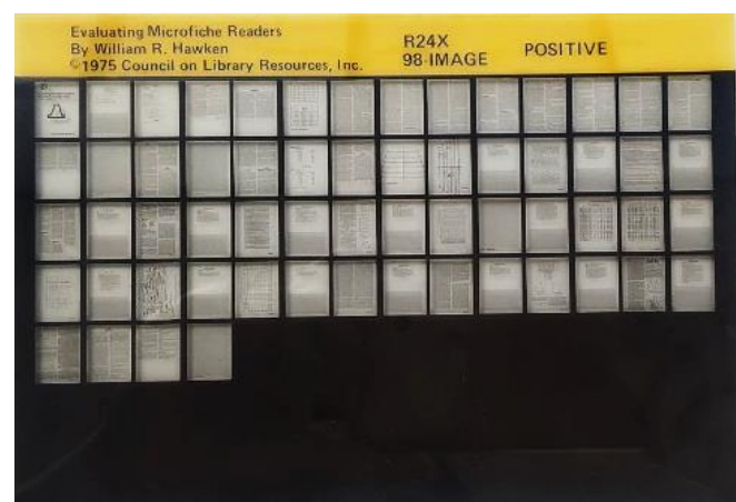
Figure 1. An example of a positive microfiche, of physical dimension 105mm × 148mm and a reduction ratio of 24X or 24 times, which will be used in the assessment of text legibility experiment. This material comes from Ref. [14].
