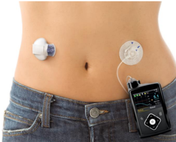
Figure 15. CSII system and CGM. Insulin pump (this particular is MINIMED® 640G) is wirelessly connected to CGM; thus, helps to ensure more accurate dosing by calculating dose based on circulating insulin levels, blood glucose levels, planned meal and personal insulin settings. Picture is reused from Medtronic website: https://www.medtronic-diabetes-mena.com/en/life-with-diabetes/managing-hypoglycaemia/insulin-pump-potential-solution with permission from Medtronic.
