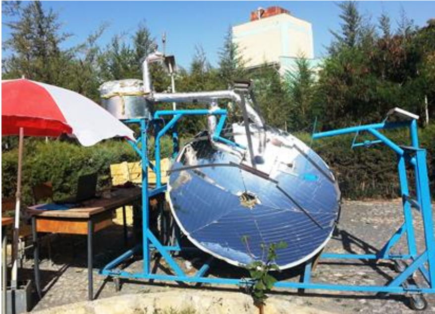
Figure 7: 1.8m parabolic dish collector with PCM storage (Mekelle Unit)
