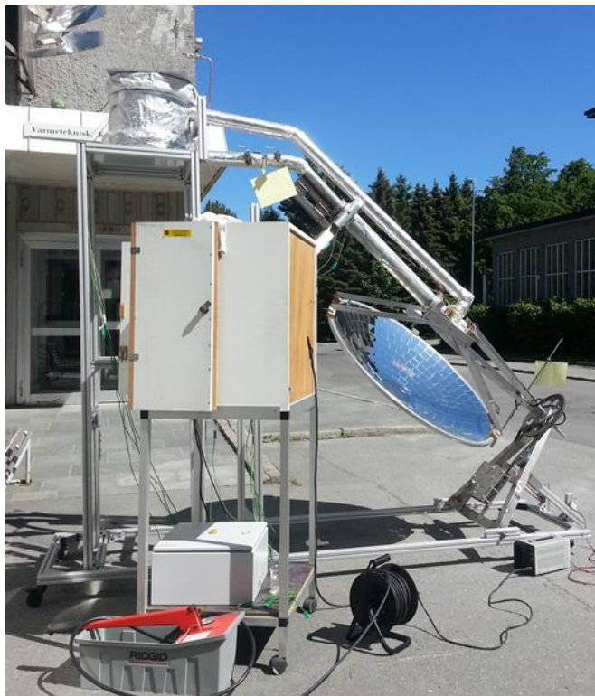
Figure 6: 1.2m parabolic dish with PCM storage (Trondheim unit)
