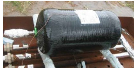
Figure 6: Experimental Type IV tank (Zalosh and Weyandt 2005)
