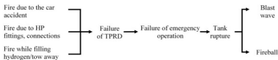
Figure 5: Tank rupture events (Dadashzadeh, Kashkarov et al. 2018)
