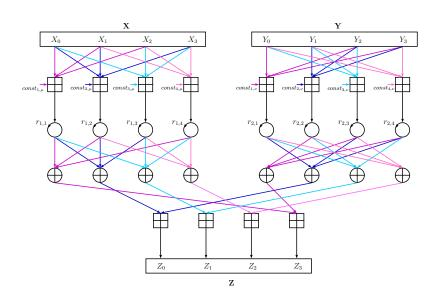
Fig. 7: Graphical representation of the ARX operation \*.
