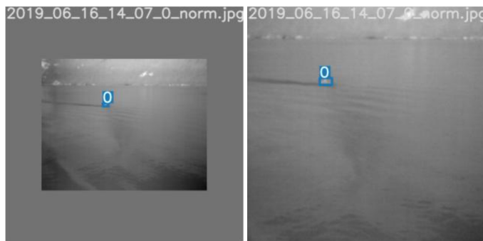
Figure 7.3: Example of a scaled image where the first is scaled down and the second is scaled up with ground truth annotation scaled correspondingly. The label 0 signifies "boat".
