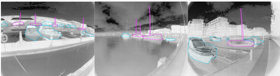
Figure 6.7: Example images from the collected Nidelva dataset with instance segmentations and class labels. Pink is "sailboat with sails down", blue is "motorboat"
