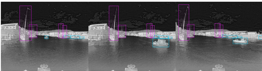
Figure 6.8: Example images from the collected milliAmpere dataset with bounding box annotations and class labels. Pink is "sailboat with sails down", blue is "motorboat".
