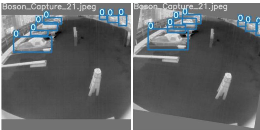
Figure 7.2: Example of the original and rotated image with ground truth annotation rotated correspondingly. The label 0 signifies "boat".
