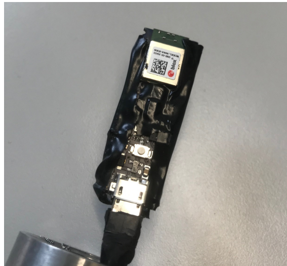
Figure 92: Arduino with electrical tape.
