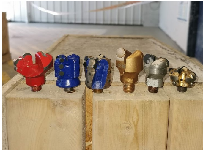
Figure 13: Different bit designs tested on the rig. The blue bits are designed by the student team and produced by Lyng Drilling.
