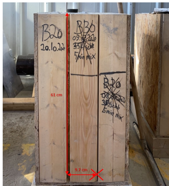
Figure 60: Exit hole displacement measurement without azimuth orientation[12].
