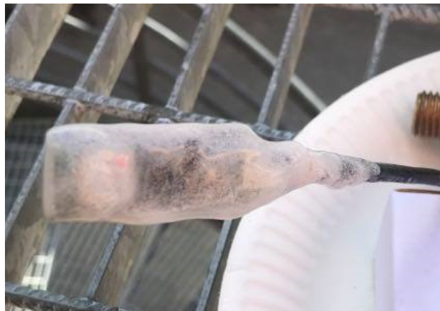
Figure 35: Arduino and USB cable with multiple layers of Plati Dip.
