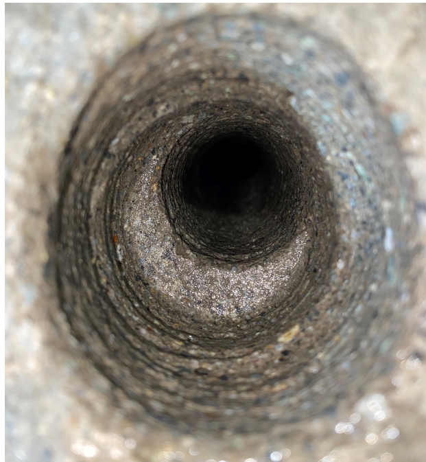
Figure 65: Autonomously drilled vertical section.
