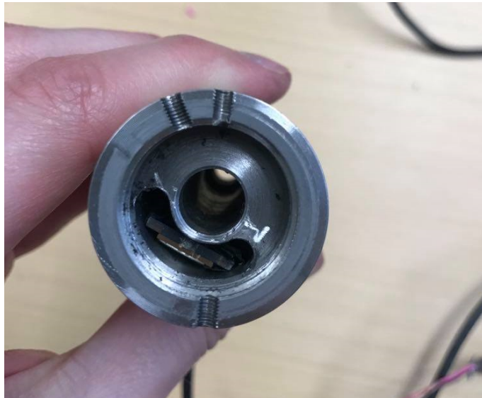
Figure 34: Inserted sensor package without epoxy.
