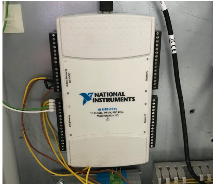
Figure 22: DAQ with connected inputs from load cell, torque sensor, and pressure transmitter.
