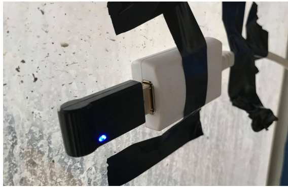
Figure 23: Bluetooth sender and receiver connected to an USB extender.
