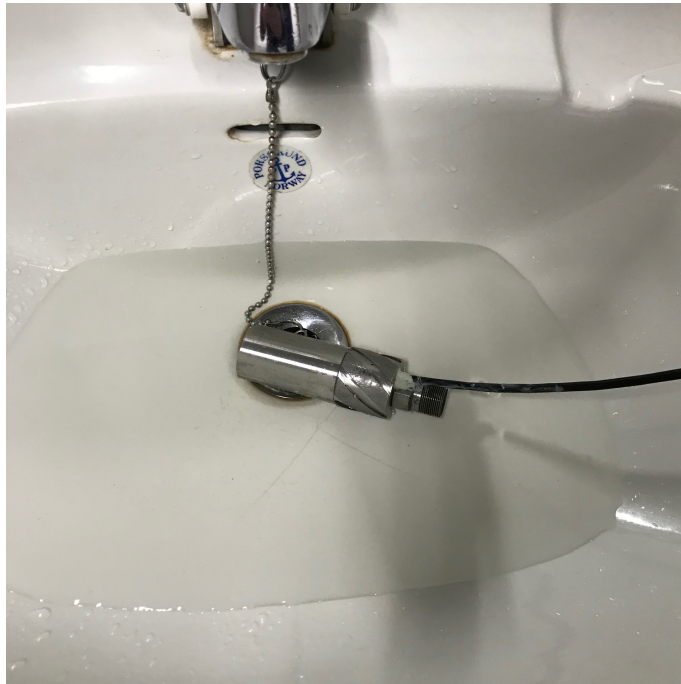
Figure 93: Submerging test of epoxy application.
