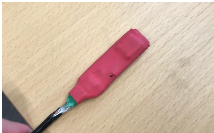
Figure 94: Arduino with shrinking tube.
