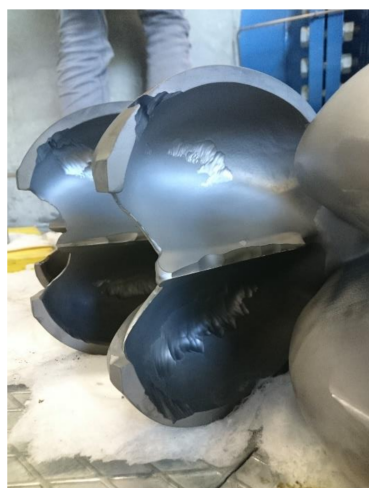
Figure 1. A Pelton turbine with severe sediment wear.
