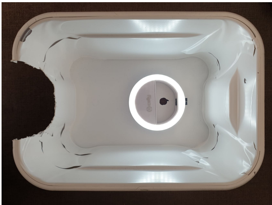
Figure 3.1.3: The box used for obtaining homogeneous light condition and fixed distance and angle to the hand. Note that this image was taken months after data collection, and that at the time of data collection, the interior painting of the box was not damaged.
