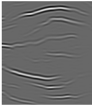
Figure 2.3.3: Gabor filtered image. The desired lines we wish to segment is separated from the background by dark ridges.
